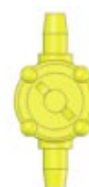
Valve is Partially Open (Reduced Flow)
